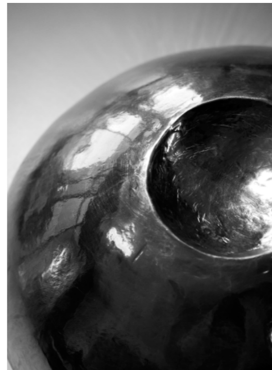
A hand worked aluminium bowl. Originally 3mm sheet aluminium. This was the first time I had ever beaten anything from metal.
